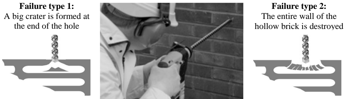
Fig. 1. Typical failures that may occur when drilling hollow bricks by a rotary hammer drill designed for drilling concrete
