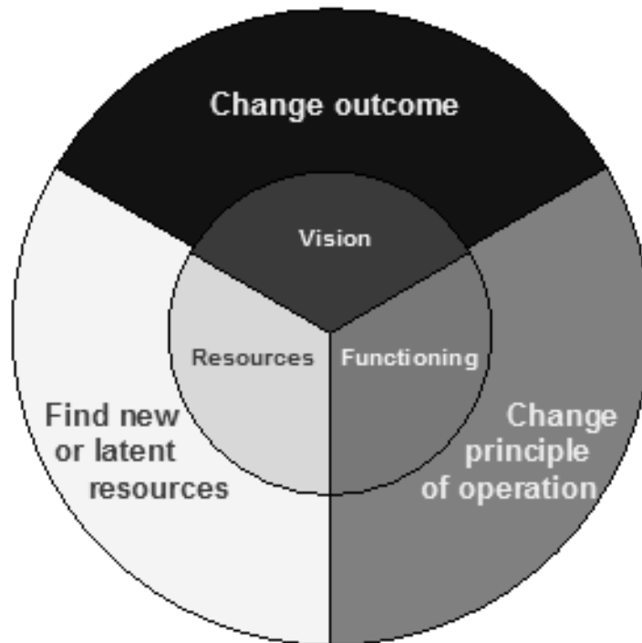
Figure 6. Categories of Inventive Principles for Changing Outcome, Changing Functioning, and Utilizing Resources for a Given System Function 22
